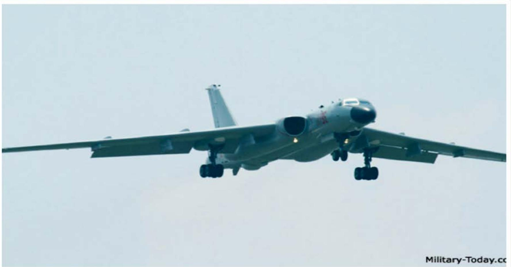
The H-6K can carry under its wing pylons six conventional or nuclear armed CJ-10A cruise missiles with 2,200 KM range. Although the H-6 was first domestically produced in 1968, this upgraded version, using composite materials, modern avionics and a powerful radar, first entered service only in October 2009.
