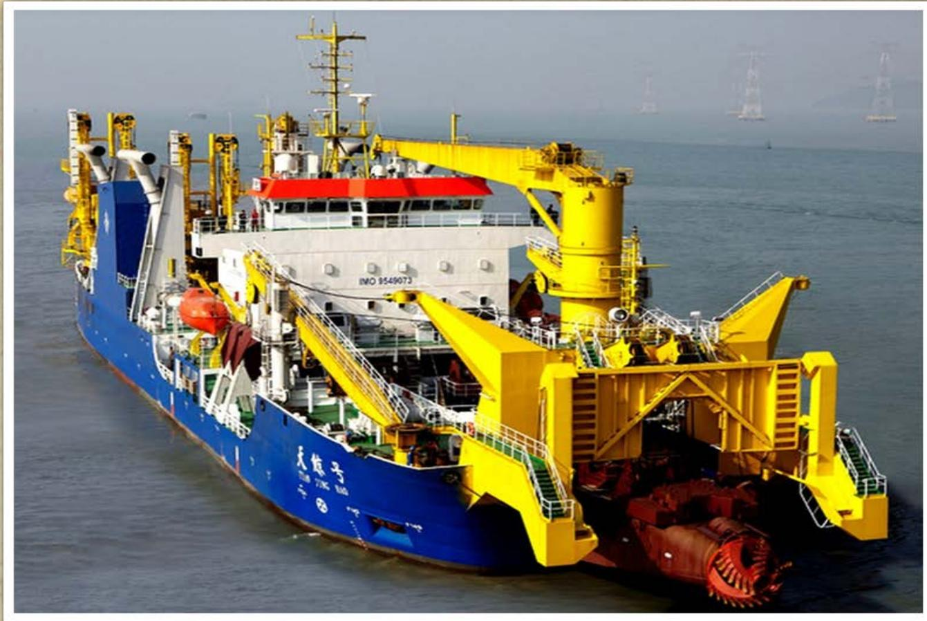
The *Tiang Jing Hao* dredger, a 127 meter-long seagoing cutter suction dredger designed by the German engineering company Vosta LMG. At 6,017 gross tons, this dredger is the largest in Asia.
