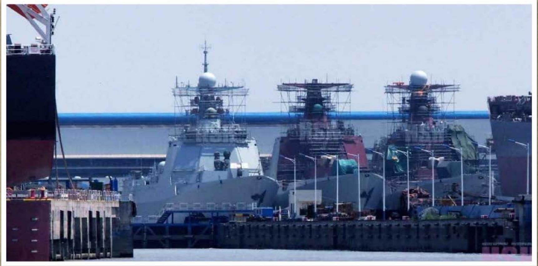
The 3<sup>rd</sup> generation Type 052D guided missile destroyer on the left was launched in 2014. The other two will be launched in 2015. The Type 052D has 64 vertical launched cells, each with 1 to 4 missiles. It carries the YJ-12 anti-ship missile with 400 KM range. China plans to deploy 10 Type 052D destroyers. China has already 6 Type 051 and Type 052A/B/C destroyers.
